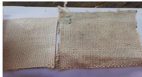
Figure: sample comparing with control sample after treating by oil staining reagent (Before treating all the fabric was stained by 1ml soybean oil)
