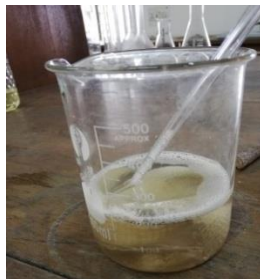
Figure: Natural Dye (Brown color) extracting from teak leaves
