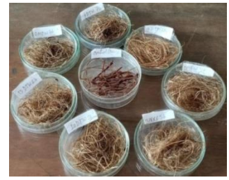
Separated fibers from dry ribbons (CVL-1)
