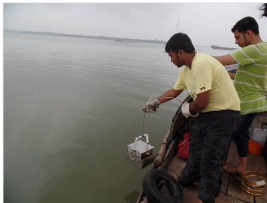
Figure 5-36: Riverbed sediment collection in the project influence area
