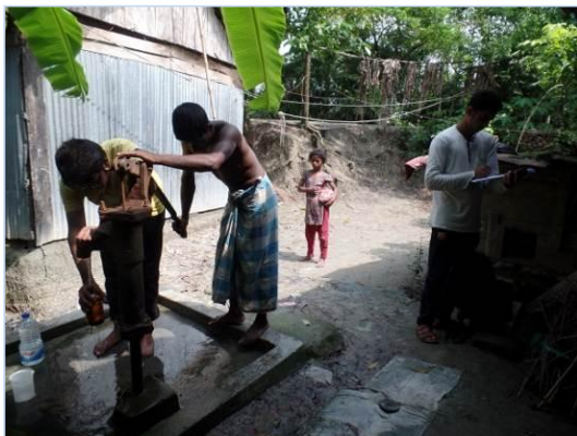
Figure 5-35: Groundwater sample collection in the project influence area
