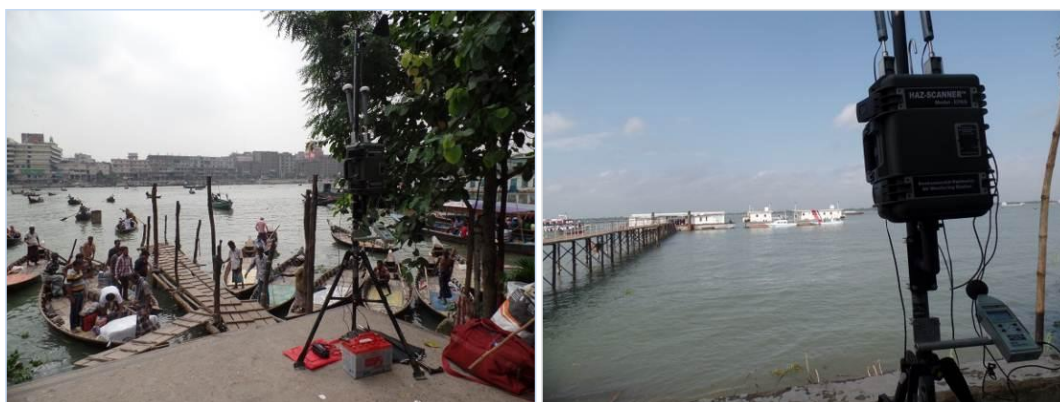
Figure 5-37: Air quality and noise level measurement in the project influence area
