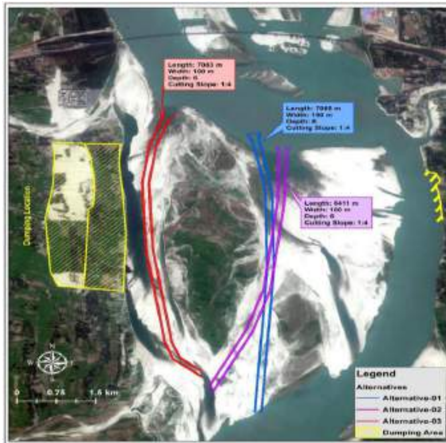
Figure 12.2: Dredging and Use of Dredged Material at Kalihati Site
