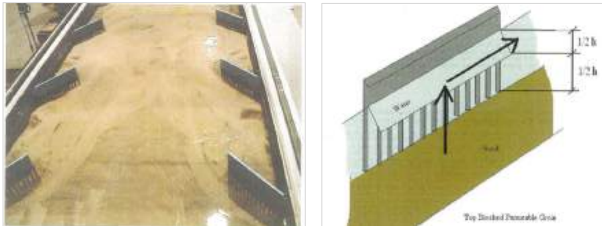
Figure 4.8: Top-Blocked Permeable Groyne (Bandal like Structure)
