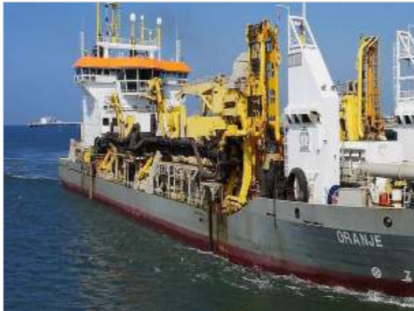
Figure 4.13: Trailing Suction Hopper Dredger
