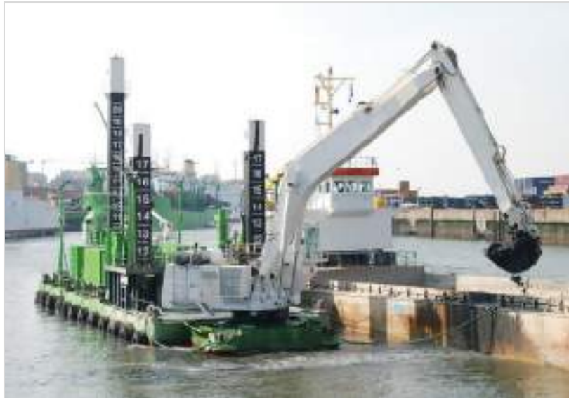
Figure 4.11: Backhoe Dredger and Barge
