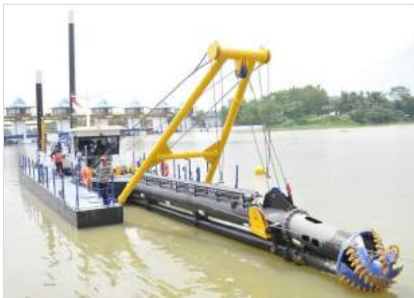
Figure 4.12: Cutter Suction Dredger
