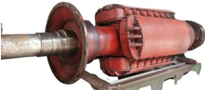
Rotor Shaft (Repairing)
