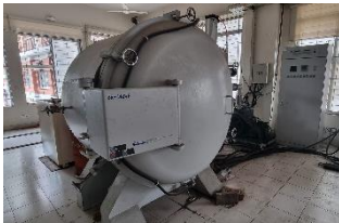
Heat Treatment Furnace
