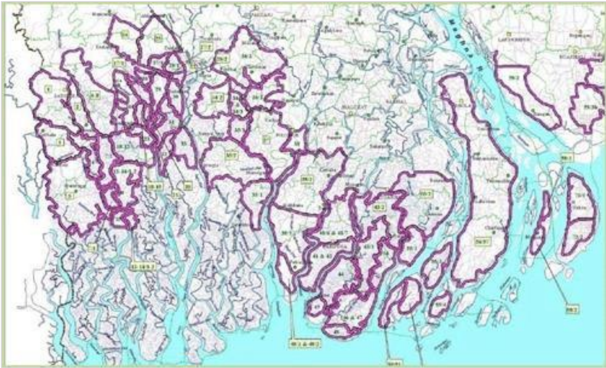
Figure 3.6: River embankments in the South West and Southern Region of Bangladesh 21
