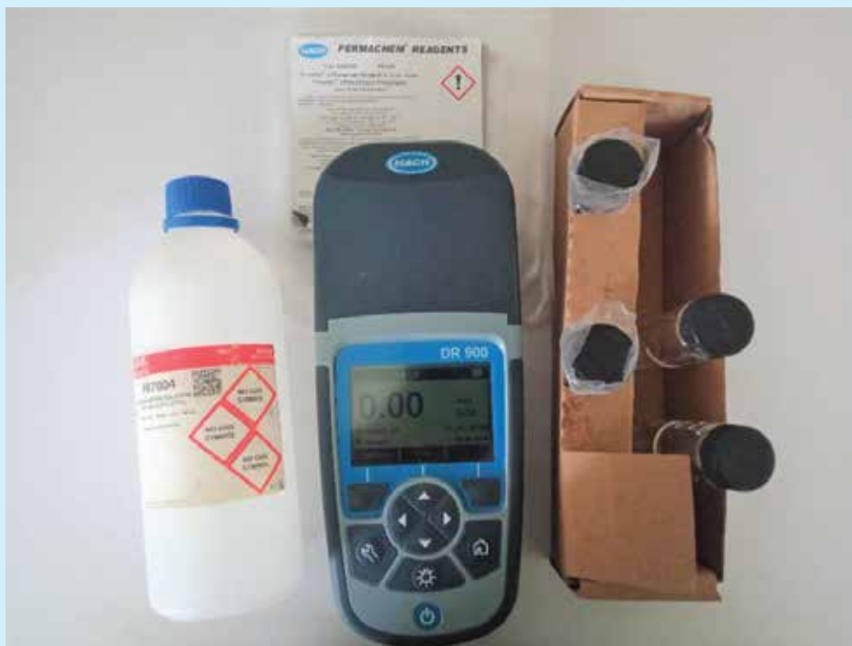
Figure 9. Colorimeter (HACH, DR 900).
