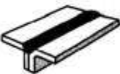
(f) Single-flare V-groove weld
