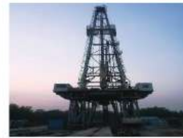
Bijoy-10 (ZJ70DBS) VFD Drive (AC-AC Type) 2000 HP 5000+ m China 2010
