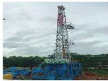
Gardner Denver E-1100 (Electrical DC-DC-Type) 1100 KW 4500 m USA 1987
