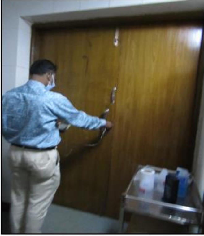
Dose Measurement of Entrance Door of PET-CT Room of Institute of Nuclear Medicine & Allied Sciences (INMAS), Dhaka.
