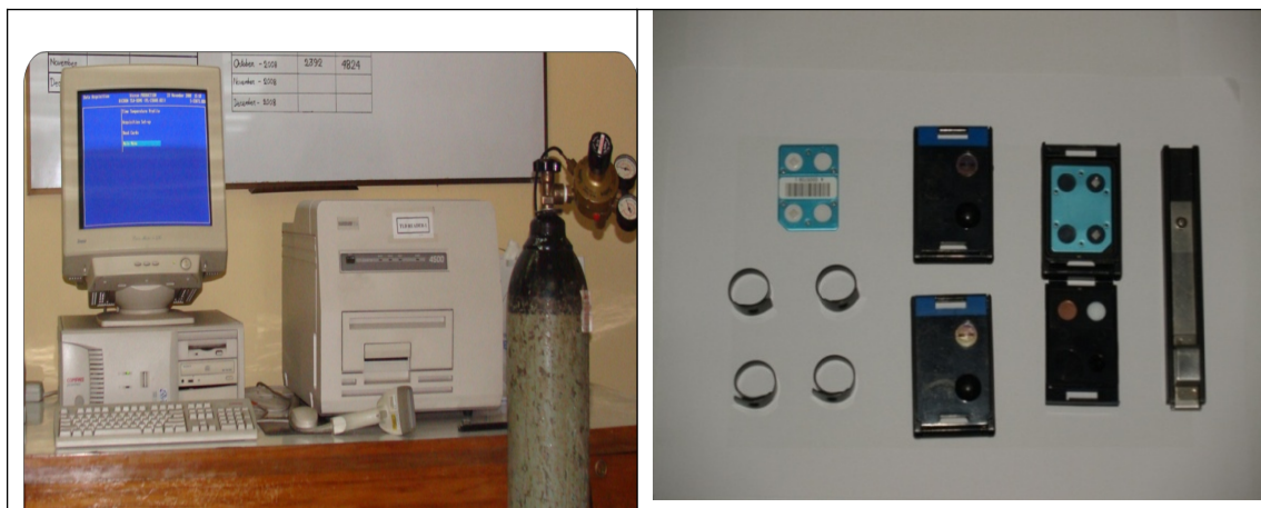
Fig.1 (a) Measuring TLD Card with Harshaw Model 4500 TLD Reader, (b) TLD Cards, Holders, Opener, ring dosimetry
