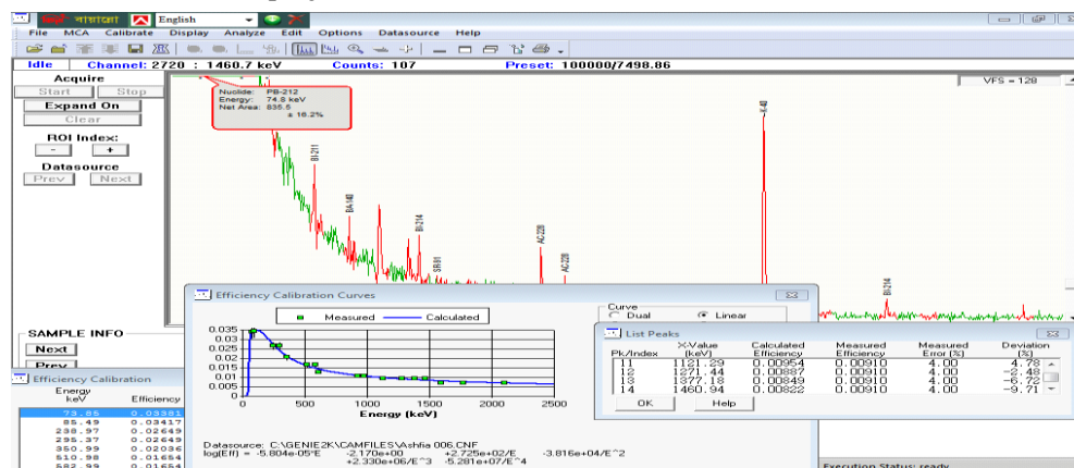
Figure: Detected gamma energy lines of radionuclides & their counting efficiency curve.
