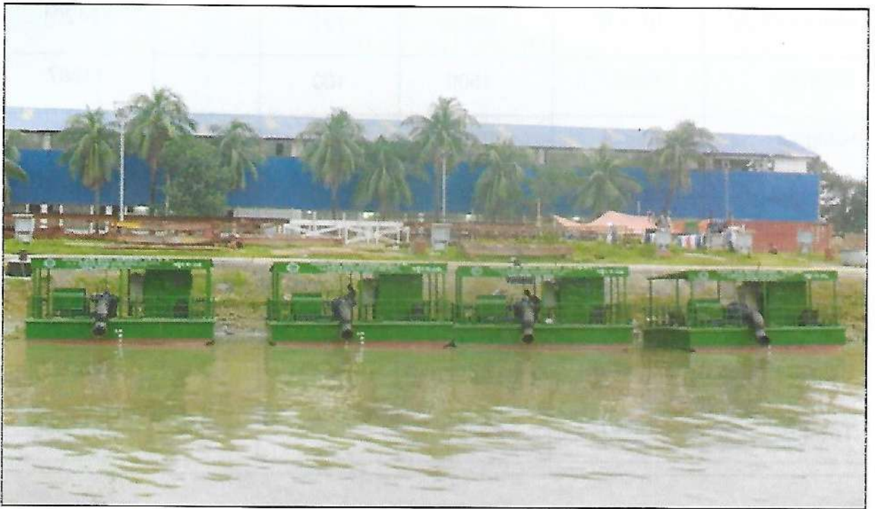
Figure 32: 12.5 Cusec Floating Pump, Dockyard Narayanganj.
