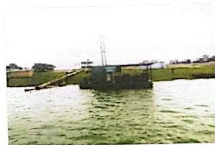
Figure 40: 25 Cusec Floating Pump at Netrokona by BADC
