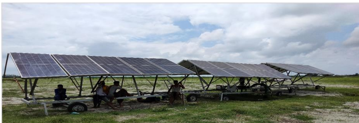
Figure 4.49: Portable Solar system for STW operated by BADC at Char area of Rangpur
