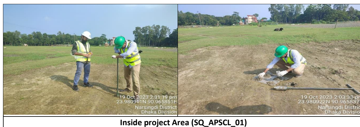
Figure 5-11: Soil Sampling Collection at Project Influenced Areas
