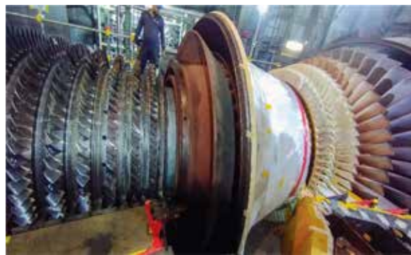
Rotor placed on Bearing
